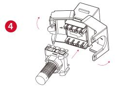
Insert the cable through the termination cap ensuring the cap fits just on the end of where the cable is stripped back to, untwist the four pairs and fan out. Following the colour code on the cap, insert the wires into their designated slots. Double check the wires are in the correct positions and then trim off the excess
