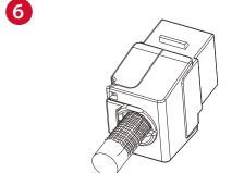
Push the termination cap down and then close the wings
